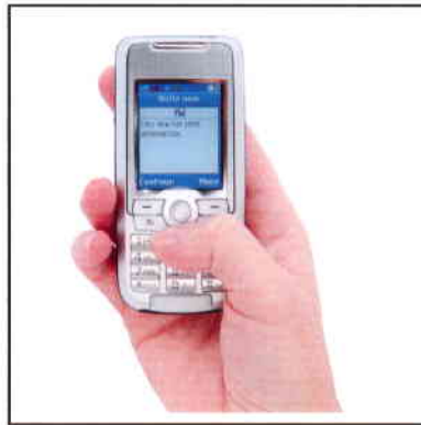
cell phone can be worn on agent or from a distance up to 40' away
